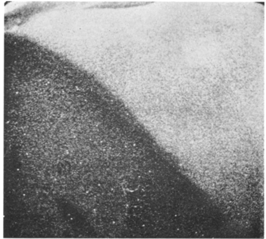
Figure 1 Accelerating voltage 20 kV. Soda-lime glass, brighter side exposed to air glow discharge for 15 min ( \times 18 ).
